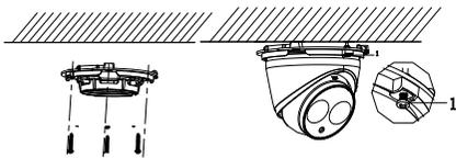
Figure 2-5 Fix the camera to the ceiling
