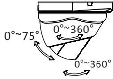
Figure 2-3 3-axis Adjustment
