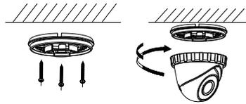
Figure 2-7 Fix the Mounting Base and Camera
