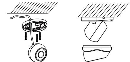
Figure 2-2 Fix the Mounting Base and the Camera
