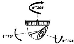
Figure 2-8 3-axis Adjustment
